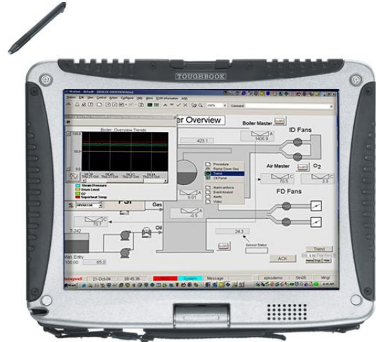
Mobile Station loaded on to a tablet PC (Panasonic Toughbook in this example).
