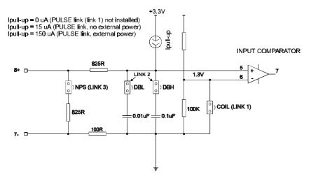
SIMPLIFIED FREQUENCY INPUT CIRCUIT
