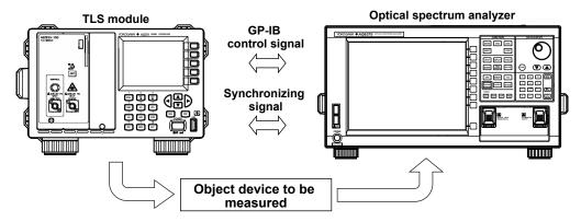
You can configure a synchronous sweep system consisting of TLS module and optical spectrum analyzer with AQ6370C and without use of personal control.
