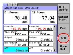
**5.** Move the cursor using the arrow keys to Enable or Disable, and press the **OK** soft key or **ENTER**.
