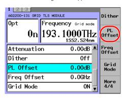
**4.** Change the numeric value with the numeric keypad or the arrow keys, and press the **OK** soft key or **ENTER**.
