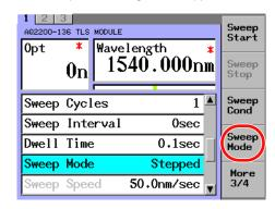
**2.** Move the cursor using the arrow keys to Continuous, and then press the **OK** soft key or **ENTER**.
