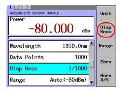
**4.** Move the cursor using the arrow keys to a desired number of decimal places and press the **OK** soft key or **ENTER**.
