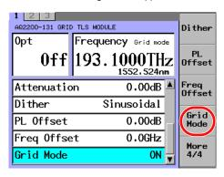
4. Use the arrow keys to select On or Off, and press the **OK** soft key or **ENTER**.
