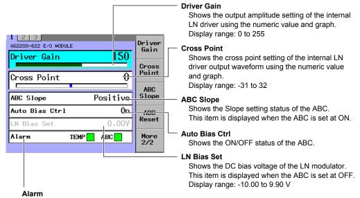
The alarm status of the module is detected and it is shown.
