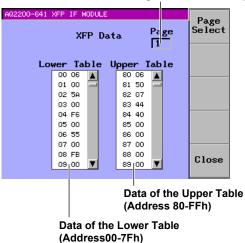
The lower and upper tables are scrolled together. You can scroll the memory data display area using the arrow keys ( $\blacktriangle \nabla$ ).
