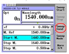
**2.** Use the arrow keys to move the cursor to a setup item, and press **ENTER**. A dialog box for entering a value appears.
