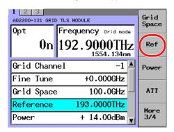
4. Use the +Grid Space or -Grid Space soft key to change the value and press the OK soft key or ENTER. You can also change the value using the numeric keypad and the arrow keys.
