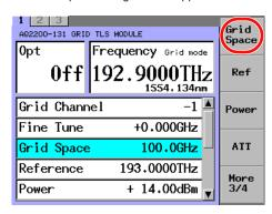
4. Use the arrow keys to select Grid Space, and press the OK soft key or ENTER. Use the arrow keys to select the spacing you want to set, and press the OK soft key or ENTER. If you select Manual, proceed to step 5.
