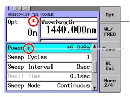
"\*" indication in the "Opt" field is the logical OR of non-achievement of the level and non-execution of the calibration. This shows that the output level in the "Power" setting field is smaller than a display level of +6.9 dBm at a wavelength of 1440 nm.
