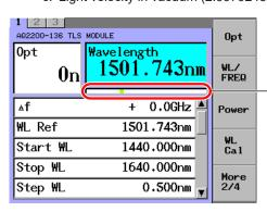
By synchronizing with the value in the "Wavelength" field, the current wavelength is shown by the bar.
