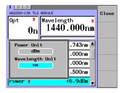
**3.** Scroll the dialog box display with the arrow keys to move the cursor to nm or THz, and then press the **OK** soft key or **ENTER**.
