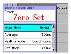
When the ZERO-SET is completed, the screen is returned to the previous screen.
