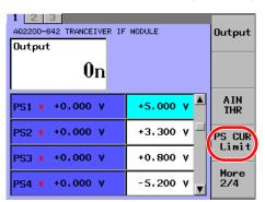
4. Use the arrow keys to move the cursor to the transceiver power supply (PS1 to PS5) whose current consumption limit you want to set, and press ENTER. A numeric input dialog box appears.
