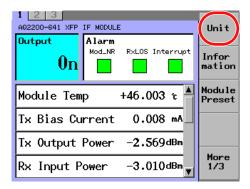
4. With the arrow keys, move the cursor to either On or Off, and press the **OK** soft key or ENTER.
