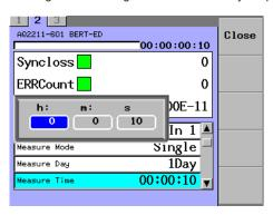
**5.** Change the numeric value with the numeric keypad or the arrow keys, and then press the **ENTER**.
