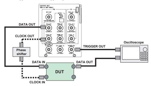
Error trigger is used as reference clock of optical transceiver.
