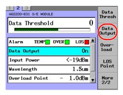
**4.** With the arrow keys, move the cursor to either On or Off, and press the **OK** soft key or **ENTER**.
