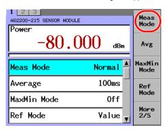
**4.** Move the cursor using the arrow keys to a desired measurement mode and press the **OK** soft key or **ENTER**.
