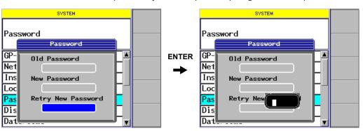
Press the Set soft key or ENTER.The new password setup is then completed.
