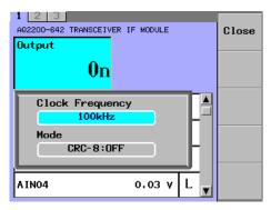
**5.** Use the arrow keys to move the cursor to 100 kHz or 400 kHz, and press the **OK** soft key or **ENTER**.
