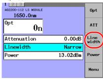
Move the cursor using the arrow keys to the line width more suitable for the purpose and press ENTER.
