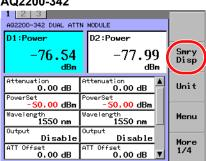
5. On the AQ2200-331/332, move the cursor using the arrow keys to ATT or Pset (ATT, Pset, or PMonitor on the AQ2200-342), and press the **OK** soft key or **ENTER**.
