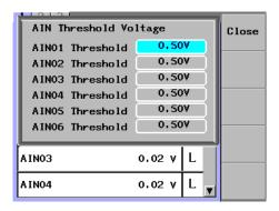
**5.** Use the numeric keypad or the arrow keys to change the value, and press **ENTER**.
