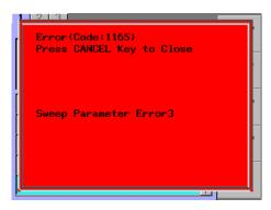
If the Step wavelength is changed after the sweep speed has been detected automatically, the automatically detected value becomes invalid.
