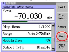
4. Move the cursor using the arrow keys to a desired mode and press the OK soft key or ENTER.
