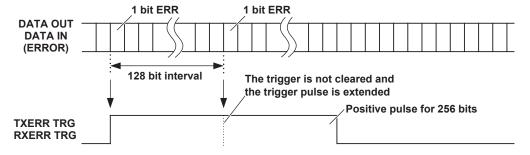
The timing of the 128-bit interval is arbitrarily determined inside the unit.
