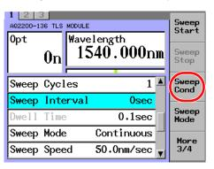
On the dialog box, input a desired numeric value through the numeric keypad or with the arrow keys, and then press ENTER.
