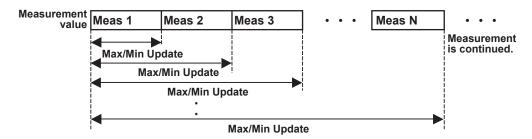
Window: The maximum value, minimum value, and (maximum value - minimum value) are calculated from the measurement values of sample quantity specified in "Data Points". For data, the latest measurement value is taken to update the measurement value while disposing of the oldest measurement value.
