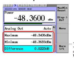
The current values are shown in the "Maximum" and "Minimum" fields, and then the value in the "Difference" field is cleared.
