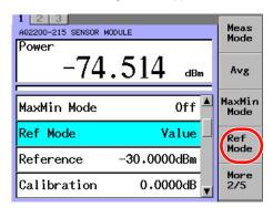
4. Press the Value x-y-z soft key to switch between Value and x-y-z.
