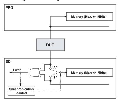
This synchronization method does not have any reference pattern. A pattern to be used as reference is made from the receive pattern and it is compared with the next receive pattern.
