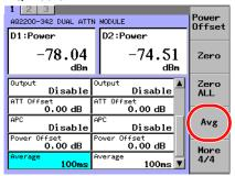
**5.** Move the cursor to a desired average time with the arrow keys, and press the **OK** soft key or **ENTER**.
