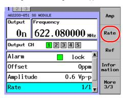
Use the arrow keys to move the cursor to 1/1 or 1/4, and press the OK soft key or ENTER
