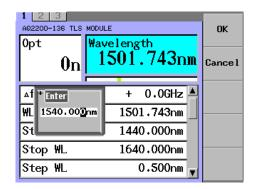
**2.** Use the numeric keypad or the arrow keys to change the value, and press the **OK** soft key or **ENTER**.
