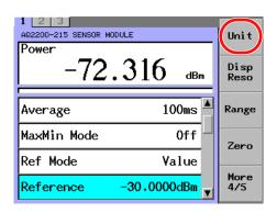
**7.** Move the cursor to using the arrow keys a desired display unit and press the **OK** soft key or **ENTER**.
