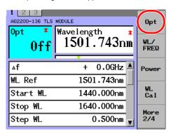
2. Move the cursor using the arrow keys to ON.
