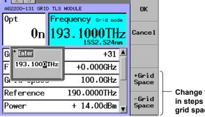
Change the frequency in steps of the specified grid spacing.
