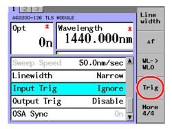
**2.** Move the cursor using the arrow keys to Ignore, and then press the **OK** soft key or **ENTER**.
