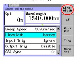
2. Move the cursor using the arrow keys to Linewidth, select the desired line width with the cursor.
