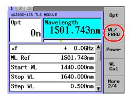
**2.** Input a desired numeric value through the numeric keypad or with the arrow keys, and then press **ENTER**.
