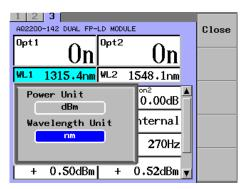
**5.** Move the cursor using the arrow keys to either of nm (wavelength display) or THz (frequency display) and press **ENTER**.
