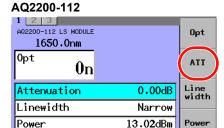
**4.** Change the numeric value with the numeric keypad or the arrow keys, and press **ENTER**.
