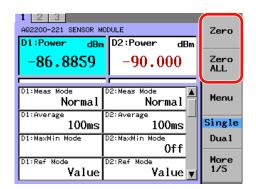
The character, Zero Set, appears while the ZERO-SET is being performed. When the ZERO-SET is completed, the screen is returned to the previous screen.
