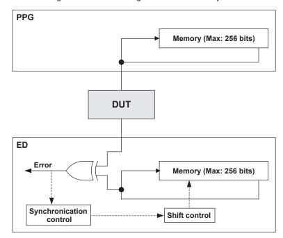
The reference pattern is compared with the receive pattern. If these patterns are not matched, the pattern is shifted one bit and it is compared with the reference pattern. This bit shift is performed repeatedly until the receive pattern meets the reference pattern in order to establish the synchronization.
