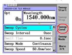
**2.** On the dialog box, input a desired numeric value through the numeric keypad or with the arrow keys, and then press **ENTER**.
