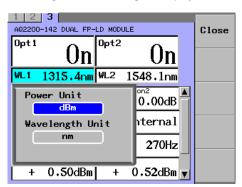
5. Move the cursor using the arrow keys to either of dBm or W and press ENTER.
