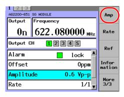
**4.** Use the arrow keys to move the cursor to 0.6 Vp-p or 1.1 Vp-p, and press the **OK** soft key or **ENTER**.
