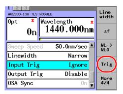
**2.** Move the cursor using the arrow keys to Sweep Start, and then press **ENTER**. Sweep Start is shown in the Input Trig field.
