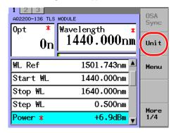
Move the cursor using the arrow keys to Power Unit, and then press ENTER. The Power display unit dialog box will appear.
