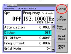
Use the arrow keys to select Sinusoidal or Off, and press the OK soft key or ENTER.
