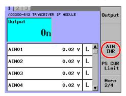
4. Use the arrow keys to move the cursor to the name of the monitor signal whose threshold you want to set (AIN01 to AIN06), and press ENTER. A numeric input dialog box appears.
