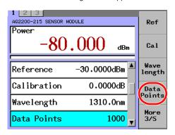
**8.** Change the numeric value with the numeric keypad or the arrow keys, and press the **OK** soft key or **ENTER**.
