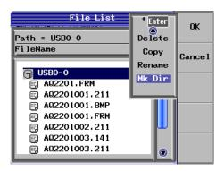
4. Use the arrow keys to move the cursor to the location where you want to create a folder, and press the Mk Dir Exec soft key.
