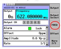
**4.** Use the numeric keypad or the arrow keys to change the value, and press **ENTER**.
