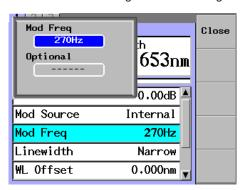
**5.** Move the cursor using the arrow keys to a desired frequency and press the **OK** soft key or **ENTER**.
