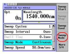
Move the cursor using the arrow keys to Manual, and then press ENTER. Manual is shown in the Sweep Mode field.
