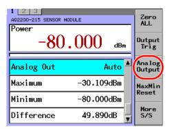
**4.** Move the cursor using the arrow keys to **Analog Out Mode** and press **ENTER**. An analog output mode selection dialog box appears.
