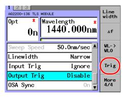
**2.** Move the cursor using the arrow keys to Step Finished, and then press **ENTER**. Step Finished is shown in the Output Trig field.
