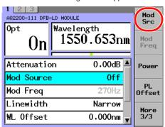
**4.** Move the cursor using the arrow keys to OFF (for CW) or Internal (for CHOP) and press **ENTER**.
