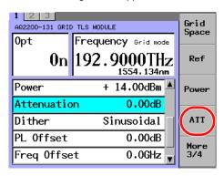
4. Change the numeric value with the numeric keypad or the arrow keys. At this time, when changing the numeric value with the arrow keys, the set value is set immediately.
