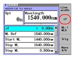
**5.** Input a desired numeric value through the numeric keypad or with the arrow keys, and then press **ENTER**.
