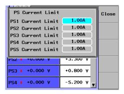
**5.** Use the numeric keypad or the arrow keys to change the value, and press **ENTER**.
