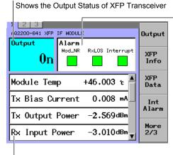
Displays the temperature inside the XFP Transceiver, the I/O optical level, and other information.
