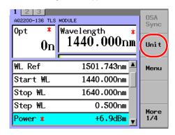
Move the cursor using the arrow keys to Wavelength, and then press ENTER. The Wavelength display unit dialog box will appear.
