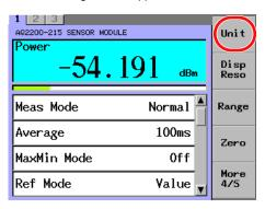
4. Move the cursor using the arrow keys to a desired display unit and press the OK soft key or ENTER.
