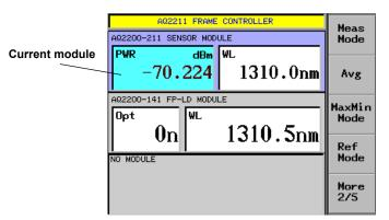
Every time the SLOT key is pressed, the current module is changed in the order of slot No.
