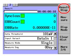
4. Press the Close soft key to close the measured results display.
