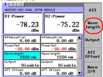
**5.** Change the numeric value with the numeric keypad or the arrow keys, and press the **OK** soft key or **ENTER**.
