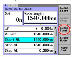
Use the numeric keypad or the arrow keys to change the value, and then press ENTER
