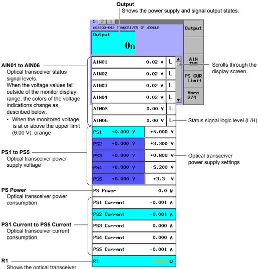
Shows the optical transceiver resistance for APS. If the resistance exceeds the measurement range, the letters are displayed using the following color.
