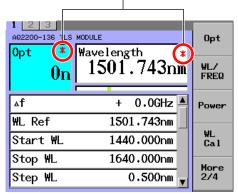
Wavelength Calibration Is Not Completed.
