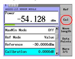
Change the numeric value with the numeric keypad or the arrow keys, and press ENTER.
