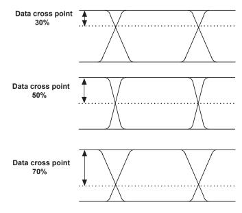
When using  $\overline{\text{DATA}}$  OUT, the signal of the cross point, that the setting ranging from 100% to set value is subtracted, is output.
