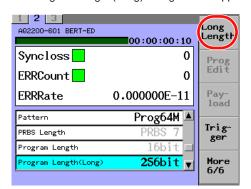
**4.** Change the numeric value with the numeric keypad or the arrow keys, and then press the **ENTER**.
