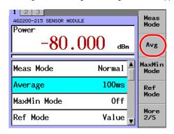
4. Move the cursor using the arrow keys to a desired averaging time and press the OK soft key or ENTER.
