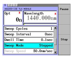
**6.** When pressing the **Cont** soft key, the temporary stop of the sweep is cancelled. Pressing the **Stop** soft key will exit the sweep.
