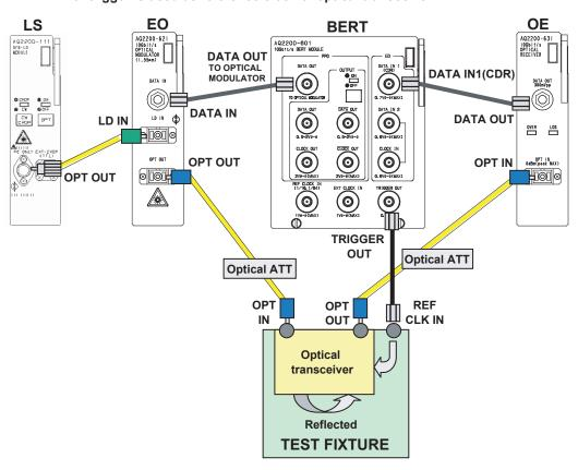
Error trigger is used as reference clock to synchronize multiple module units.
