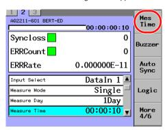
**4.** Use the arrow keys to move the cursor to the unit of time that you want to change (hours, minutes, or seconds), and press **ENTER**.
