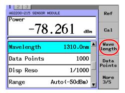
**4.** Change the numeric value using any of two operating procedures shown below and press the **OK** soft key or **ENTER**.
