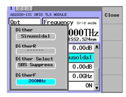
Change the numeric value with the numeric keypad or the arrow keys, and press the  ${\bf OK}$  soft key or  ${\bf ENTER}$ .
