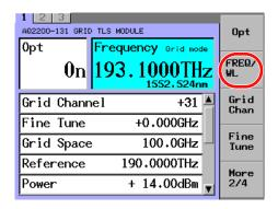
4. Use the +Grid Space or -Grid Space soft key to change the value and press the OK soft key or ENTER. You can also change the value using the numeric keypad and the arrow keys.
