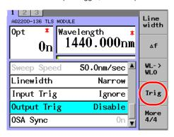
**2.** Move the cursor using the arrow keys to Sweep Finished, and then press **ENTER**. Sweep Finished is shown in the Output Trig field.
