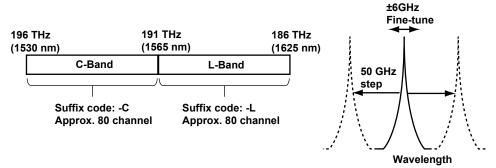
You can set the frequency in the following ranges. You can also change the unit to nm and set the value in terms of the wavelength.
