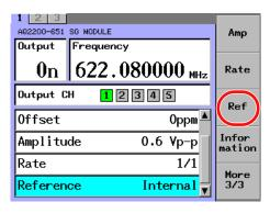
4. Use the arrow keys to move the cursor to Internal or External, and press the OK soft key or ENTER.
