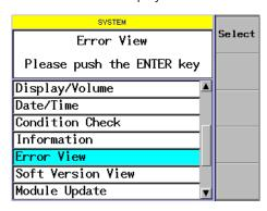
**2.** Use the arrow keys to move the cursor to Error View, and press the **Select** soft key or **ENTER**.
