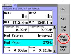
4. Move the cursor using the arrow keys to a desired frequency and press the OK soft key or ENTER.
