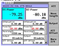
**5.** Move the cursor to a desired decimal place with the arrow keys, and press the **OK** soft key or **ENTER**.
