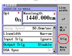
2. Move the cursor using the arrow keys to Sweep Started, and then press **ENTER**. Sweep Started is shown in the Output Trig field.
