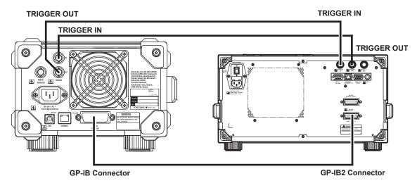
Connection Diagram for Synchronous Sweep of AQ2200-136 and AQ6370C
