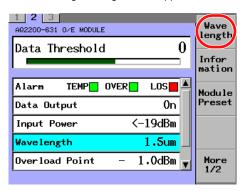
4. With the arrow keys, move the cursor to either 1.5um or 1.3um, and press the OK soft key or ENTER.
