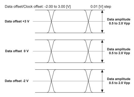
For the Clock offset, the DC offset voltage can be changed in the same manner as described above. However, the amplitude is fixed at approximately 0.60 [Vpp].
