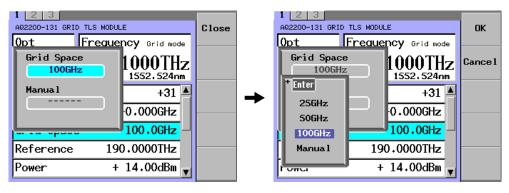
**5.** Move the cursor using the arrow keys to Manual and press **ENTER**. The Manual dialog box will appear.
