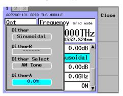
Change the numeric value with the numeric keypad or the arrow keys, and press the **OK** soft key or **ENTER**.
