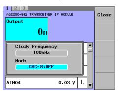
**5.** Use the arrow keys to move the cursor to CRC-8 OFF or CRC-8 ON, and press the **OK** soft key or **ENTER**.
