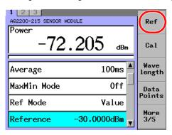
**5.** Change the numeric value with the numeric keypad or the arrow keys, and press the **OK** soft key or **ENTER**.
