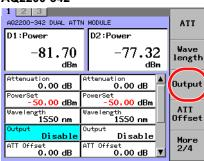
**5.** Move the cursor using the arrow keys to either of Enable or Disable and press the **OK** soft key or **ENTER**.
