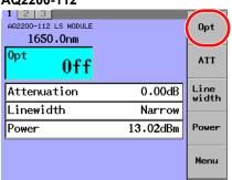
**4.** Move the cursor using the arrow keys to either of On or Off and press the **OK** soft key or **ENTER**.
