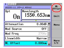
4. Change the numeric value with the numeric keypad or the arrow keys, and press the OK soft key or ENTER. Even if the unit of wavelength is THz, the wavelength offset is set in units of nm.
