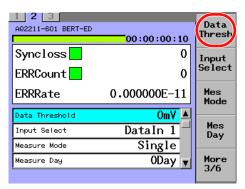
**4.** Change the numeric value with the numeric keypad or the arrow keys, and then press the **ENTER**.
