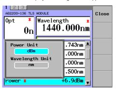
Scroll the dialog box display with the arrow keys to move the cursor to dBm or W, and then press the OK soft key or ENTER.
