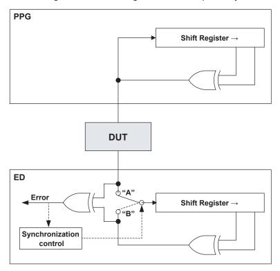
When "Auto Sync" is OFF, the switch is fixed at "B".
