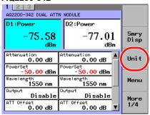
**5.** Move the cursor using the arrow keys to either of dBm or W and press the **OK** soft key or **ENTER**.
