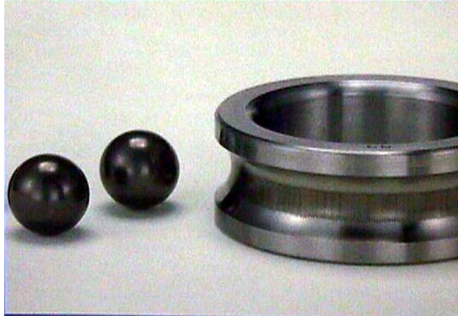
Figure 7 – Bearing Damage due to Shaft Currents
